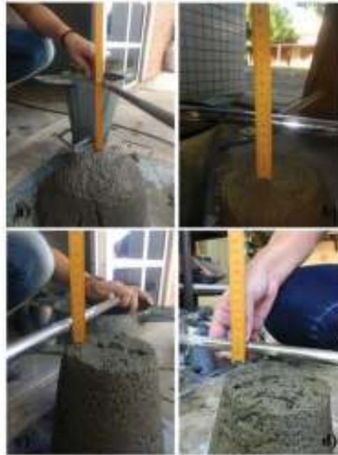
Figura 45: a) Slump T0; b) Slump T10; c) Slump T15; d) Slump T20.
